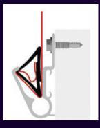
The locking keepers can then be inserted into the Poster Frame on each side.
